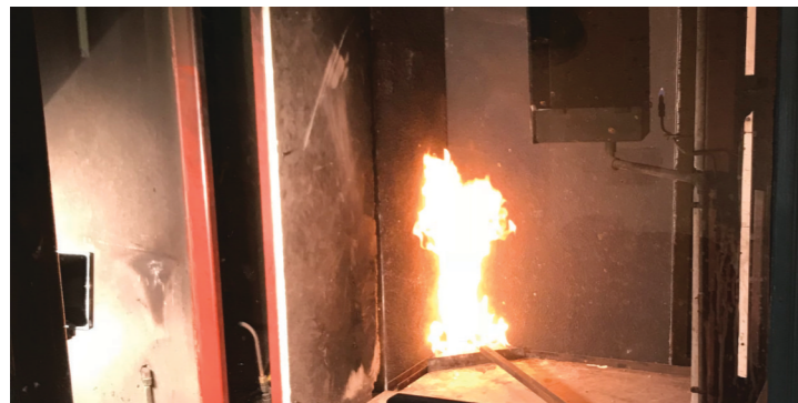
■ Photograph of EN 13823 (SBI) Testing
