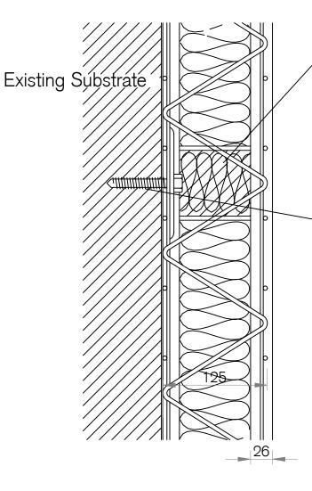
Carefully cut out existing core insulation at all fixing positions. Install fixing and washer through rear of space frame cage and replace insulation plug over fixing head.
